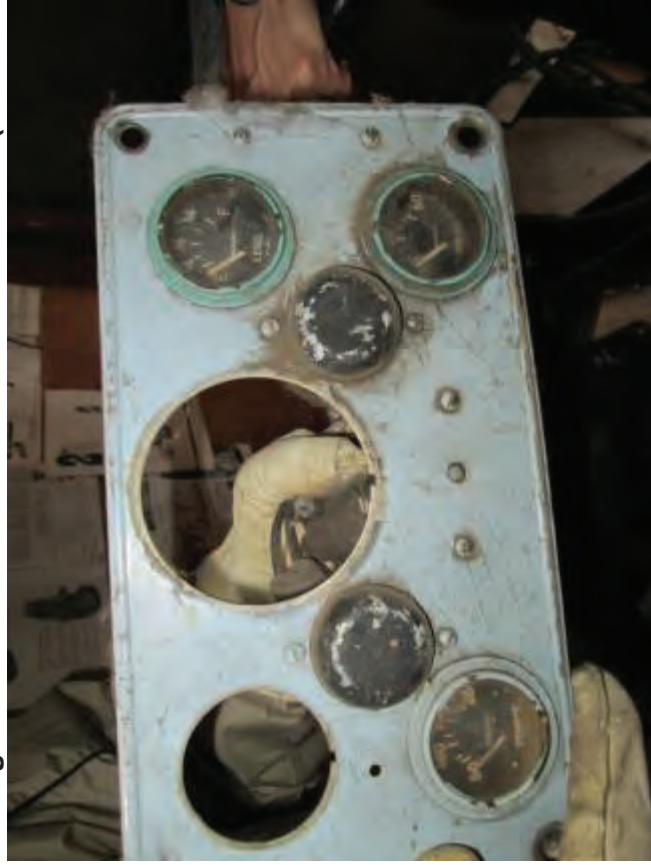
A-11. Gauges Found with Measurable Exposure Rates up to 100 \mu R/h on contact
