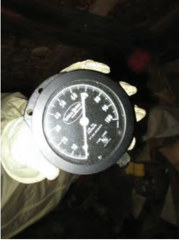
A-10. Gauge Found with up to 30,000 cpm and 16 \mu R/h on contact
