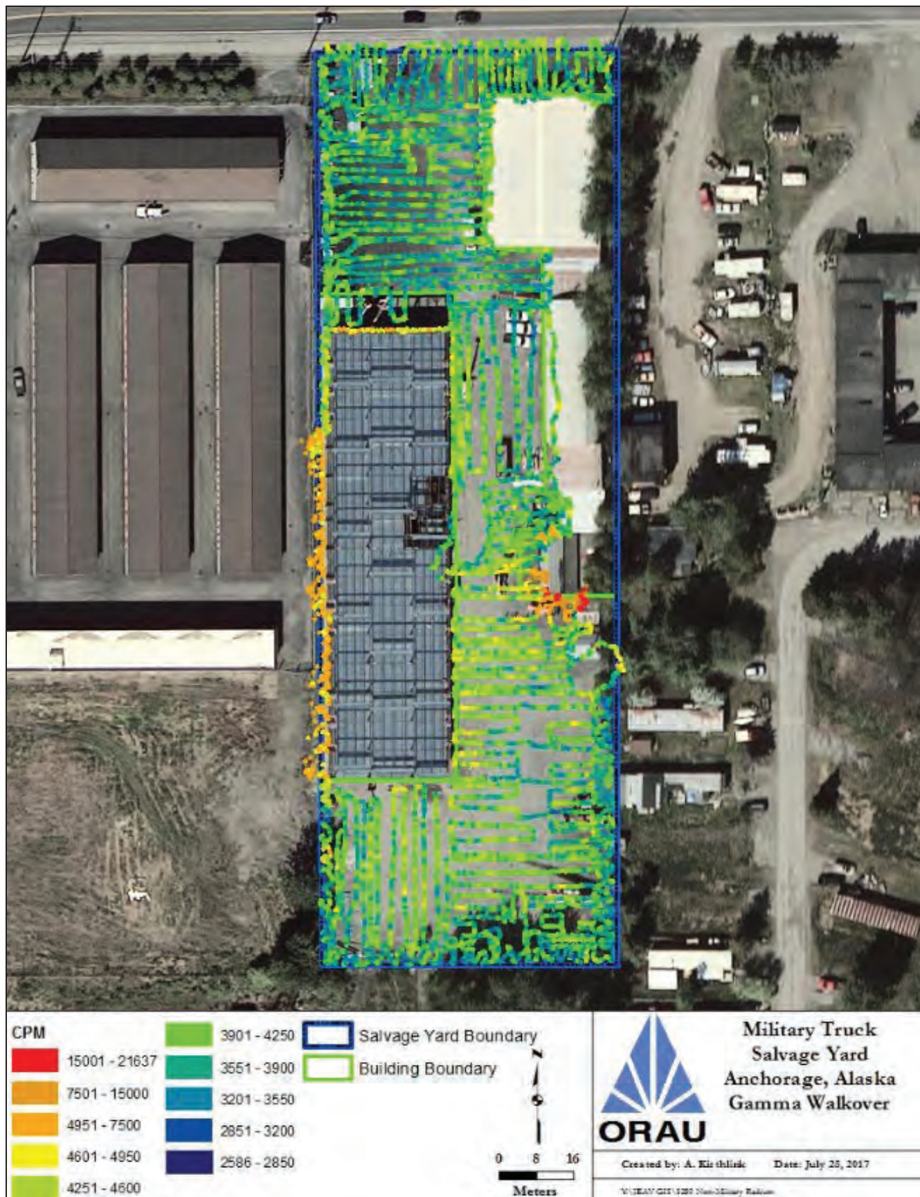
Figure B-1. Gamma Walkover Survey Data for the Land Area
