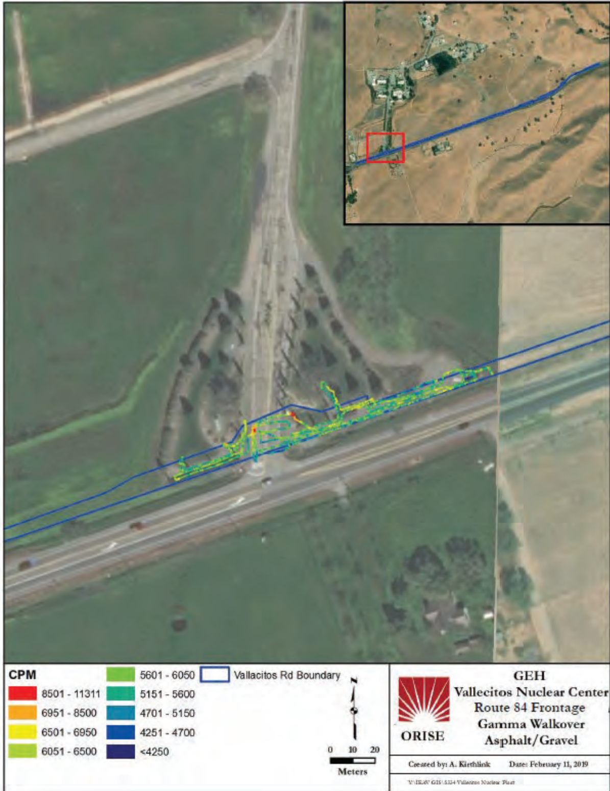
Figure A.2. Gamma Walkover Data (2 of 9) with Elevated Radiation Levels in the Landscaping
