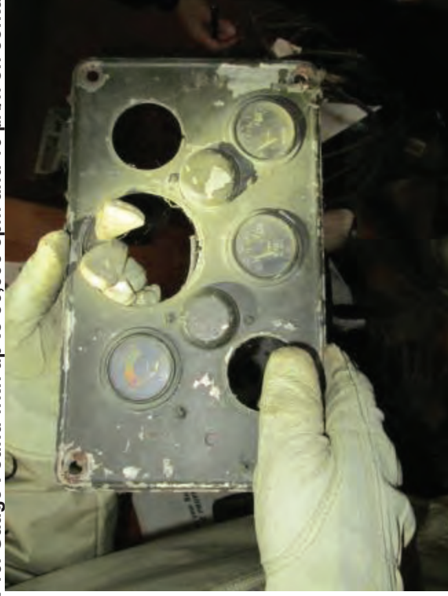
A-12. Gauges Found with Measurable Exposure Rates up to 100 \mu R/h on contact
